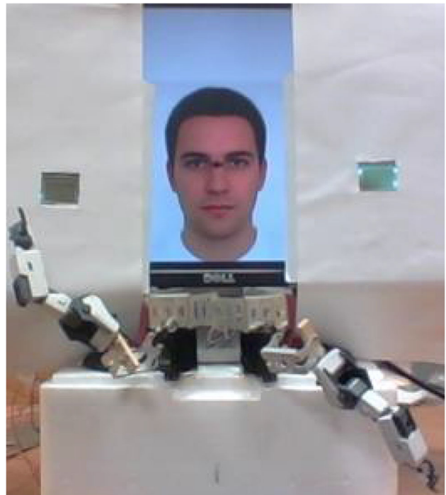
Fig. 1 Experimental setup of Experiment 1. In this example, the left robot arm is pointing to the left LED display. The static face in the middle was always the same and presented throughout all trials. The LED displays on which target letters were flashed are visible as little rectangles on the left and right side of the computer screen
