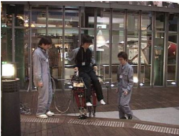
Fig. 15 WL-16R II carried a person to climb steps in Hakata Riverain shopping mall
