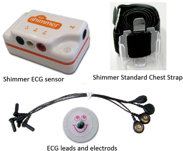
Fig. 3 Shimmer ECG sensor and related materials
