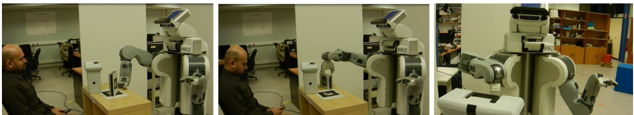
Fig. 21 Using the effect to parameter converter, learned effects of the hide task has been converted into constraints comparable with our geometric planner for human-centered tasks [51]. Using those, the PR2
