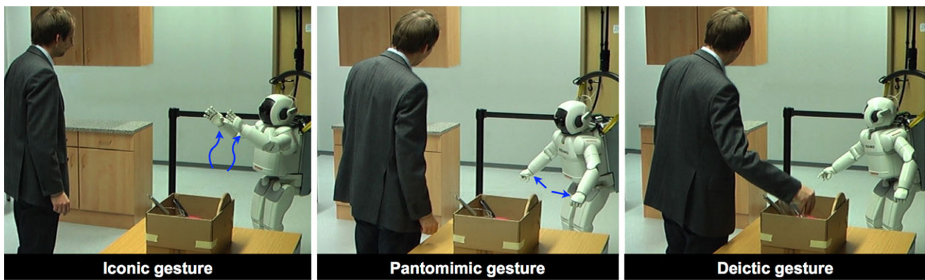
Fig. 2 Examples of the three gesture types performed by the robot in the multimodal conditions (adapted from [21]; arrows indicate the movement trajectory and direction of dynamic gestures): iconic ges-
