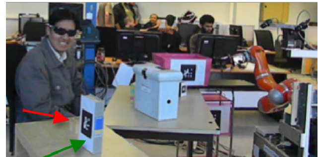
Fig. 18 Task of making an object accessible to the robot. In the absence of proactive behavior, the user is holding the object and waiting for the robot to take
