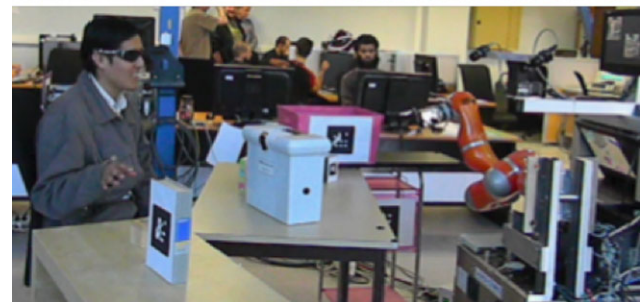
Fig. 19 Task of making an object (marked as red arrow ) accessible to the robot. In the absence of further feedback from the robot, the human is confused about which object to make accessible, as he failed to ground the object referred by the robot (Color figure online)
