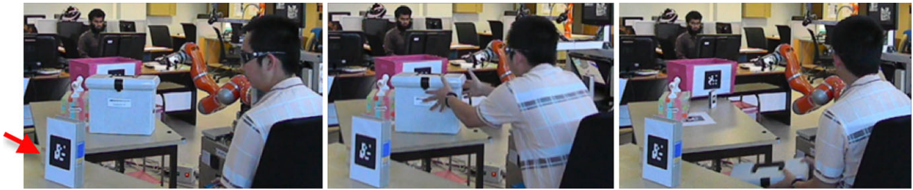
Fig. 17 Task of making an object (pointed by the red arrow ) accessible to the robot. In the absence of proactive behavior, the user took away the white box as an attempt to clear the obstruction for the robot to take the object (Color figure online)
