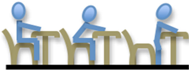
Fig. 3 Taxonomy of reach actions: (a) arm-shoulder reach, (b) arm-torso reach, (c) standing reach. (Adapted from [10, 19])
