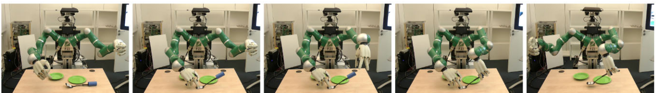
Fig. 20 Lifting a spoon: execution on Adero using online object detection to localize the spoon handle
