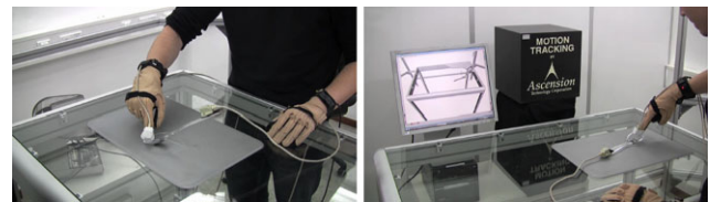
Fig. 4 Sensory environment front (left) and back (right): datagloves, motion tracker and 3d visualization. Human demonstrations to lift a spoon
