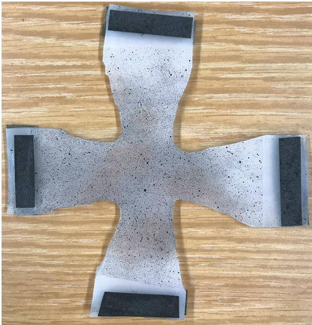
Fig. 1 Ecoflex (silicone rubber) sample after preparation for biaxial testing
