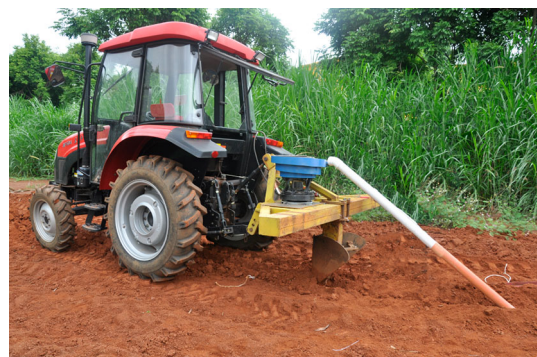
Fig. 16 Sugarcane planter with electromagnetic vibration-type single-bud sugarcane seed metering device
