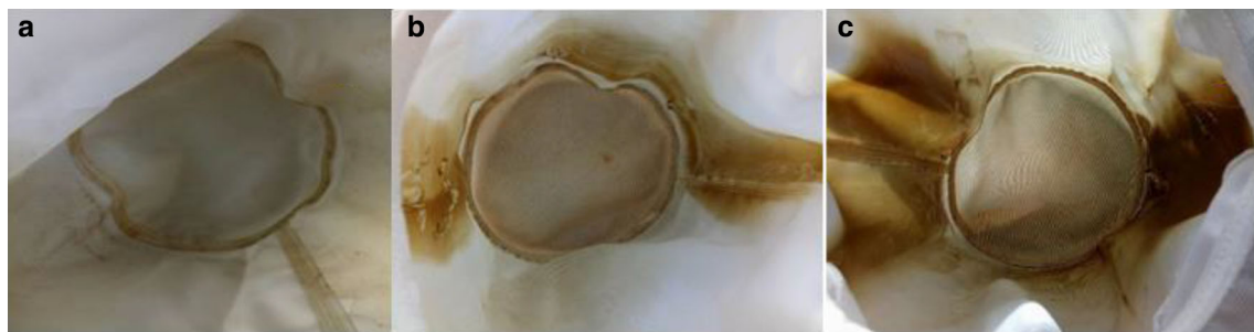
Fig. 2 Suspended insoluble mud materials from the filter bag. After filtration, the juice clarified with CaO solution to adjusted pH of the cane juice at a pH 6, b pH 7 and c pH 8.5
