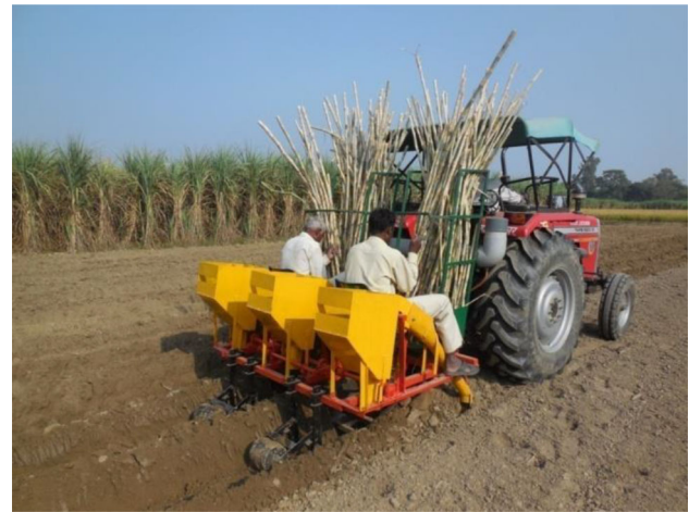
Fig. 4 Developed sugarcane-cum-potato planter in field operation
