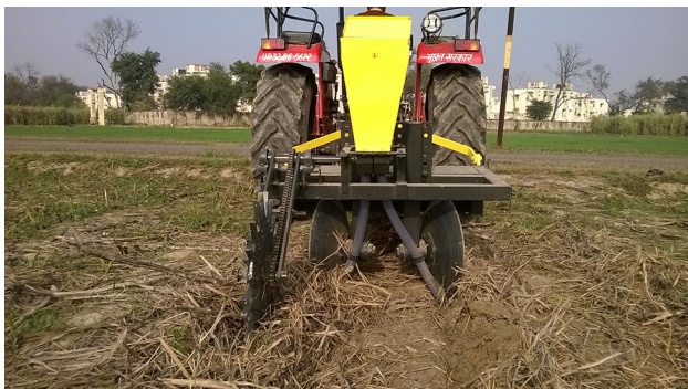
Fig. 5 Developed disc-type ratoon management device in field operation
