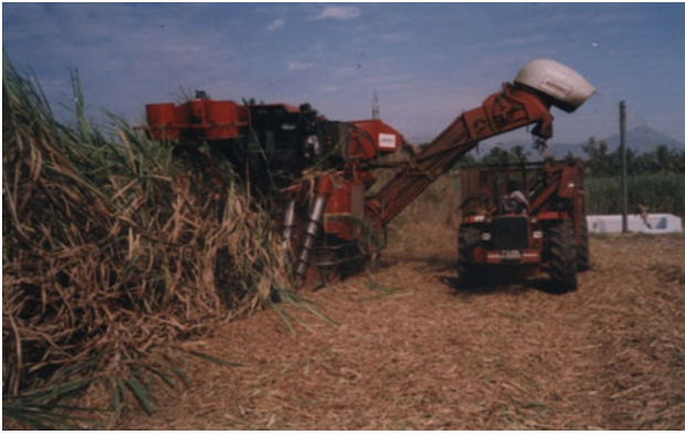
Fig. 4 Modern sugarcane chopper harvester (Austoft 7000) during trials
