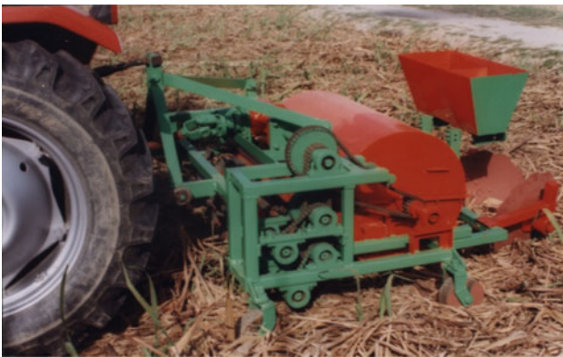
Fig. 5 IISR trash handling equipment
