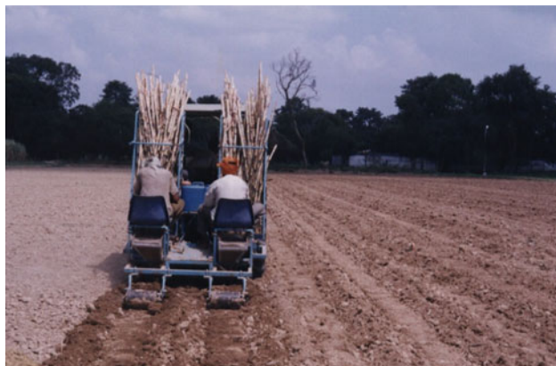
Fig. 1 IISR sugarcane cutter planter (ridger type) in operation
