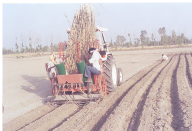
Fig. 2 IISR raised bed seeder-cum-cane planter in operation
