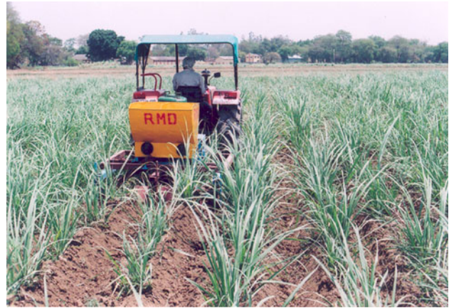
Fig. 6 IISR ratoon management device in field operation
