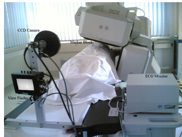
Figure 2. The respiratory gating equipment mounted on the SPECT system. The RPM system, an infrared reflective plastic box, is placed on the patient's abdominal surface and the camera with an infrared illuminator surrounding the lens is placed on the SPECT bed.
