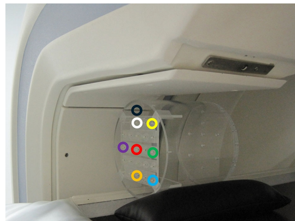
Figure 3. Throughout the axially central transverse plane, 64 sensitivity measurements were made. Additional axial sensitivity plots were made for eight transverse locations and are shown here with respect to the detector face. The locations are referred to in the text as “nearest” (black circle), “top” (white circle), “center” (red circle), “bottom” (orange circle), “top right” (yellow circle), “right” (green circle), “bottom right” (blue circle), and “left” (violet circle). In this figure only, patient left corresponds to the left side of the image.
