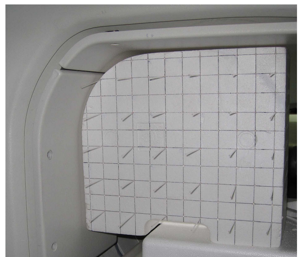
Figure 2. To map spatial resolution in air, 30 point sources were arrayed in a 5-cm grid pattern set in a polystyrene foam block, as shown here, and stepped throughout the camera FOV in 2.5-cm increments. Patient left corresponds to the left side of this image.
