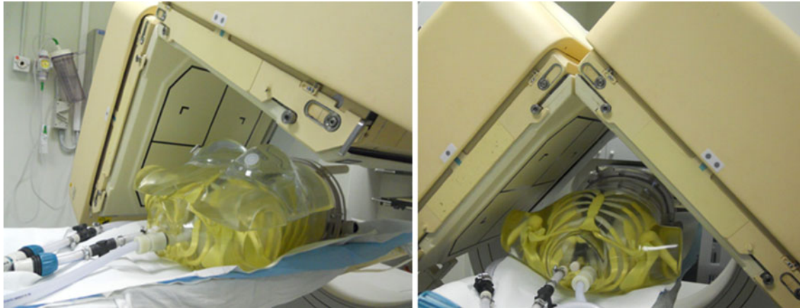
Figure 3. The large female ( left ) and the average male ( right ) body types of the anthropomorphic phantom in the Philips Forte/Vantage SPECT/ ^{153}\text{Gd} .
