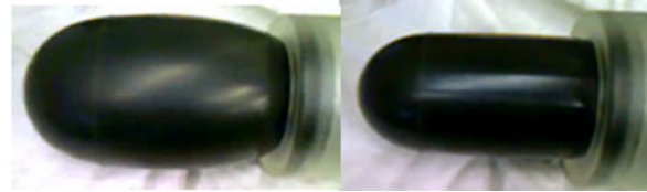
Figure 2. The cardiac phantom during expansion (diastole) and compression (systole).
