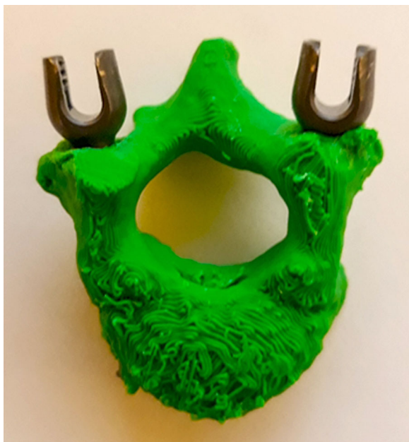
Fig. 3 Plastic model with the screws inserted using guiding templates. Properly placed screws
