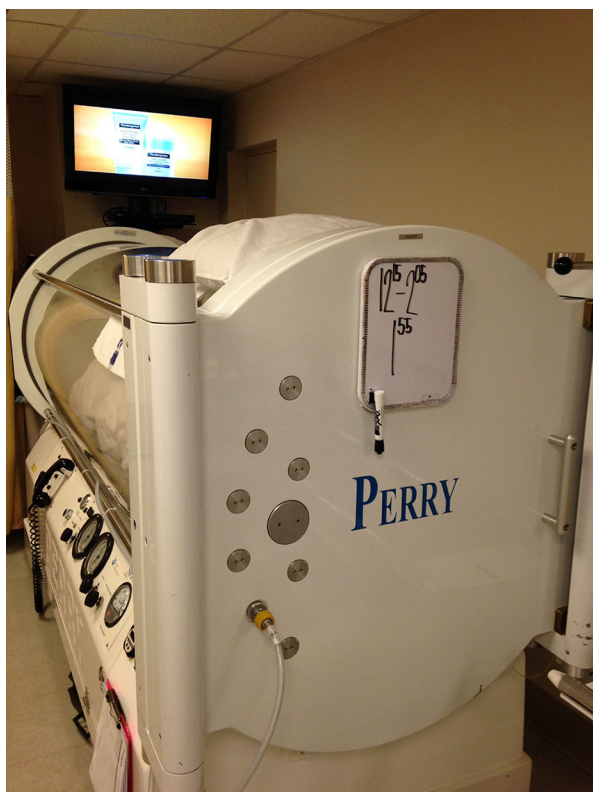
Fig. 2 Hyperbaric oxygen wound therapy chamber (Sigma 34 Hyperbaric Chamber, Perry Biomedical, Riviera Beach, FL, USA)
