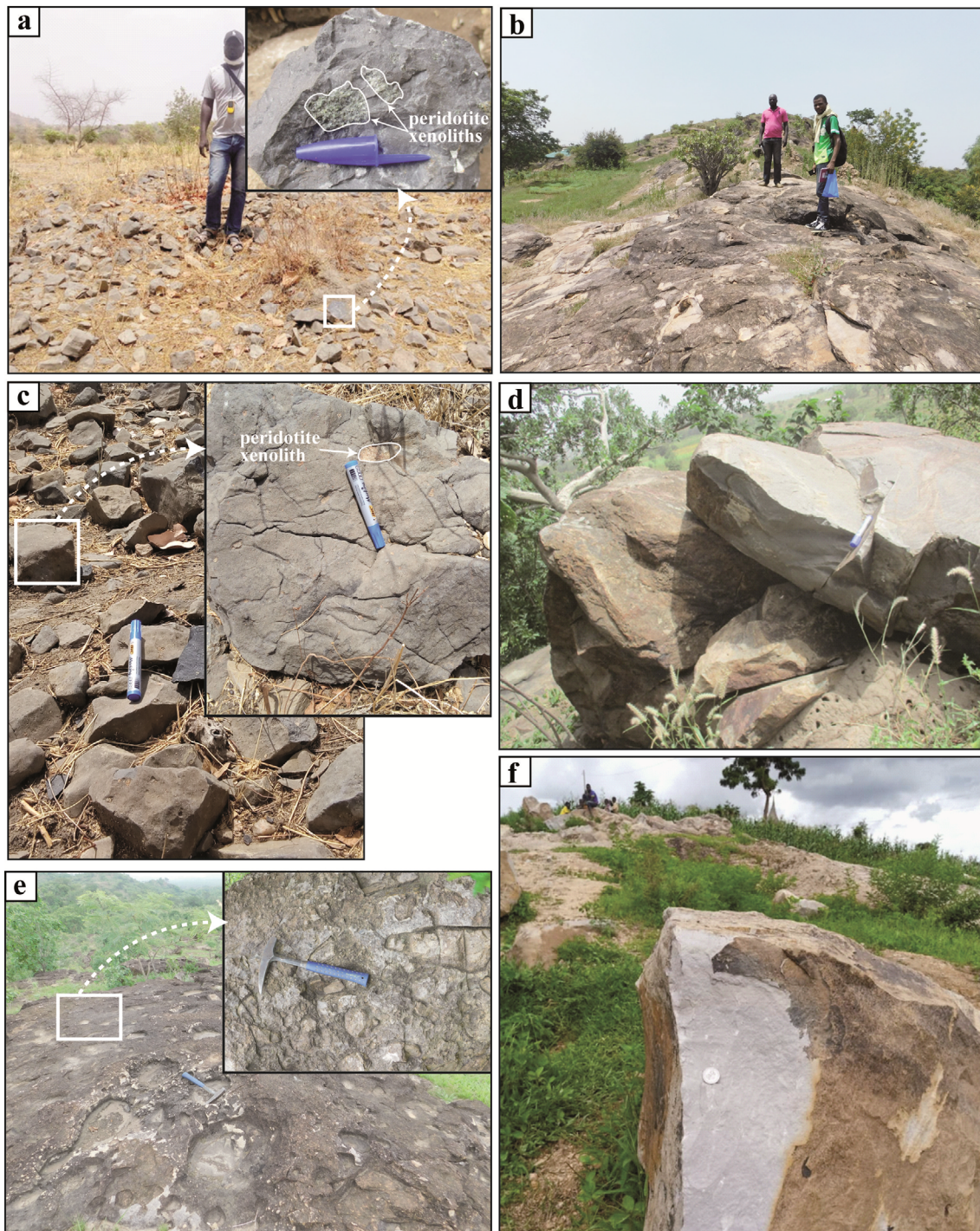
Fig. 4. Field photos of the studied lavas. (a) basanite of Udkia, the length of the pen cap is 5.5 cm, (b) trachybasalt of Ouro-Tada, (c) trachybasalt of Mandaka, the length of the marker is 14 cm, (d) Trachyte of Udkia, (e) Alkaline rhyolite of Sékandé, the length of the hammer is 33 cm, (f) subalkaline rhyolite of Kosséhône.
