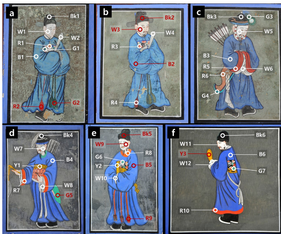
Fig. 1. Analysis points of Sungseonjeon wall paintings. (a) O1, (b) O2, (c) O3, (d) N1, (e) N2, and (f) N3. The red labels indicate the delaminated specimen collection points.
