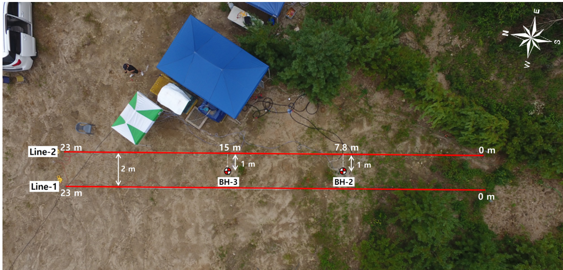
Fig. 12. Layout of boreholes BH-2 and BH-3 and the electrical resistivity survey line.
