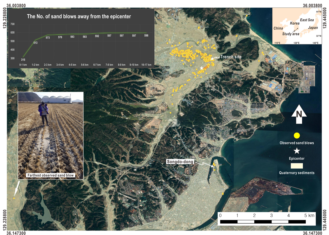
Fig. 1. Spatial distribution of the sand blows around the epicenter with the numbers of the sand blows away from the epicenter (top left). All sand blows occur only on the Quaternary sediments.
