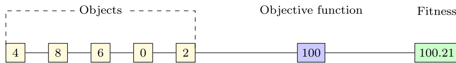
Fig. 1 An example of the chromosome design. The objects (items) packed in the knapsack are represented by their identifiers. The objective function value is calculated by summing the benefit of all the objects while the fitness is calculated according to the fitness function
