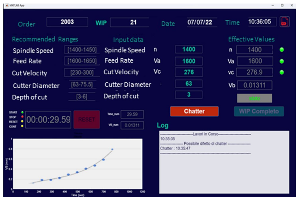
Fig. 4 Digital twin interface for milling process (Level 2)
