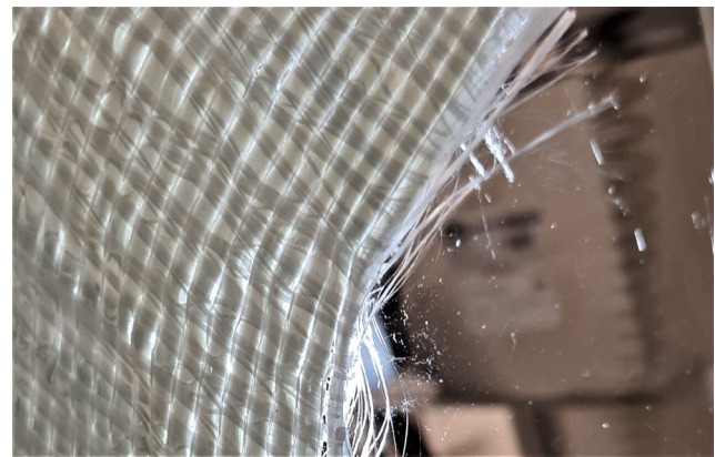
Fig. 8 Backside of fiber mat of diamond w. plates specimen at high elongation (side without edge stitching). The backing fibers remain in their place without slipping
