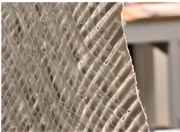
Fig. 7 Backside of the fiber mat of rectangular specimen at high elongation with slipping of backing fibers visible
