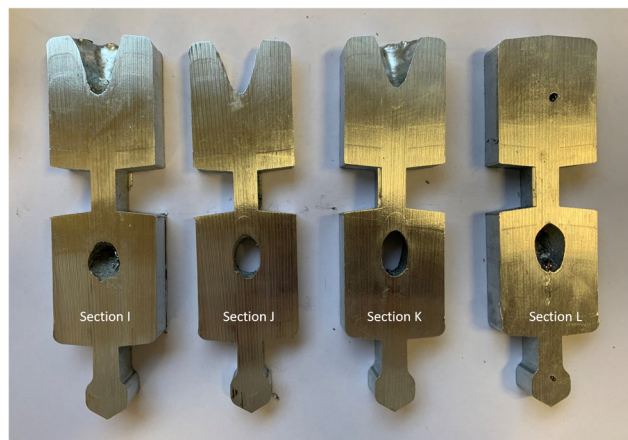
Fig. 12 Pictures of some planes showing macro-shrinkage formation
