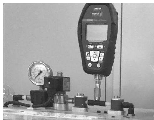
Fig. 2 Manometer for measuring the pressure
