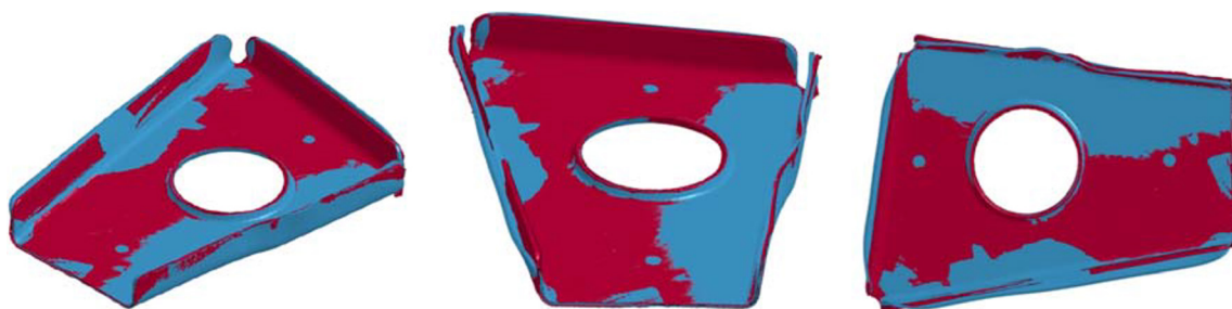
Fig. 31 Superposition of the digitized experimental deformed shape (in red) and the computed deformed shape (in blue)
