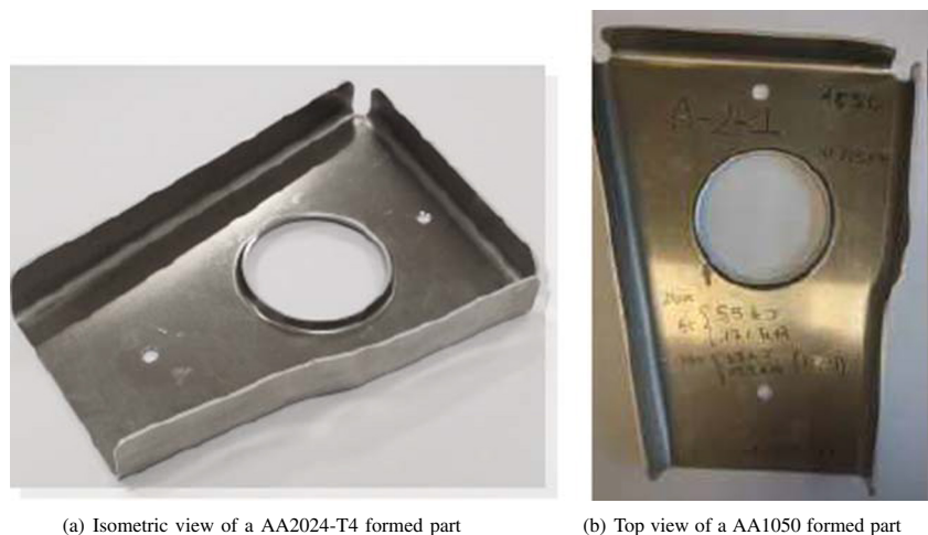
(a) Isometric view of a AA2024-T4 formed part
