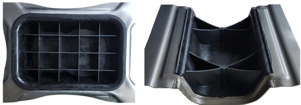
Fig. 9 Hybrid formed tub geometry and u-profile with steel (Table 1) and PA6-LGF40
