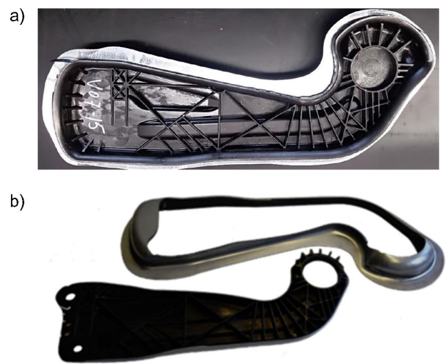
Fig 17 (a) Trailing arm produced by hybrid forming and (b) after waterjet cutting
