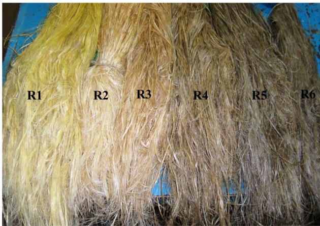
Fig. 4 Photograph of flax fibres samples with different degrees of retting. From unretted sample (R1) on the left to retted sample on the right (R6) [67]
