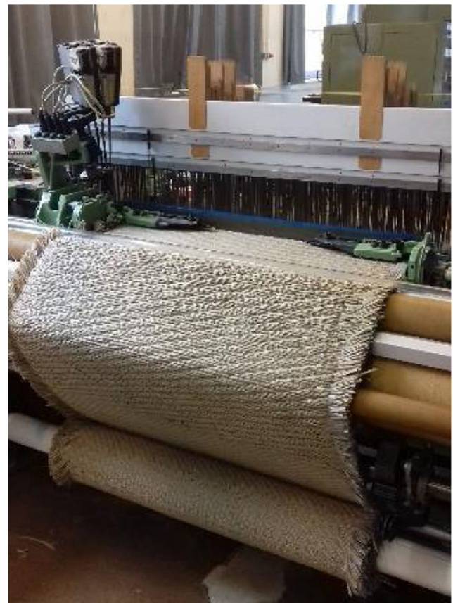
Fig. 12 Manufacture of 3D-warp interlock from flax rovings [148]
