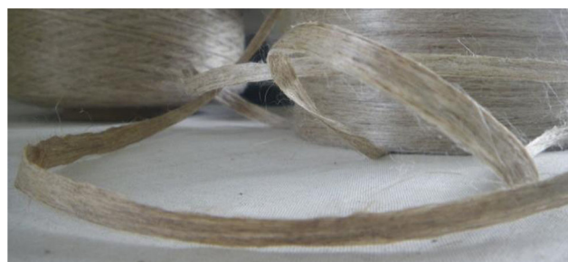
Fig. 7 Flax yarn assembled by adhesive bonding
