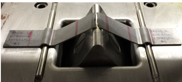
Fig. 3 Setup of an angular stretch bend test. A 25 mm wide strip of DP600 sheet steel is gripped with a ligament length of 180 mm and deformed by a punch under constant displacement control
