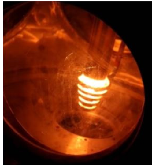
Fig. 12 Induction melting experiment with five-turn conical induction coil
