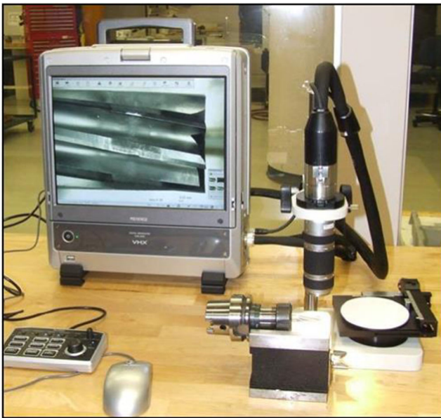
Fig. 6 Optical microscope type Keyence VHX-600 + 500F
