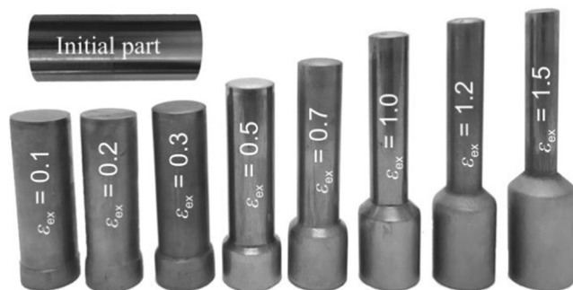
Fig. 19 Extruded parts with different extrusion strains
