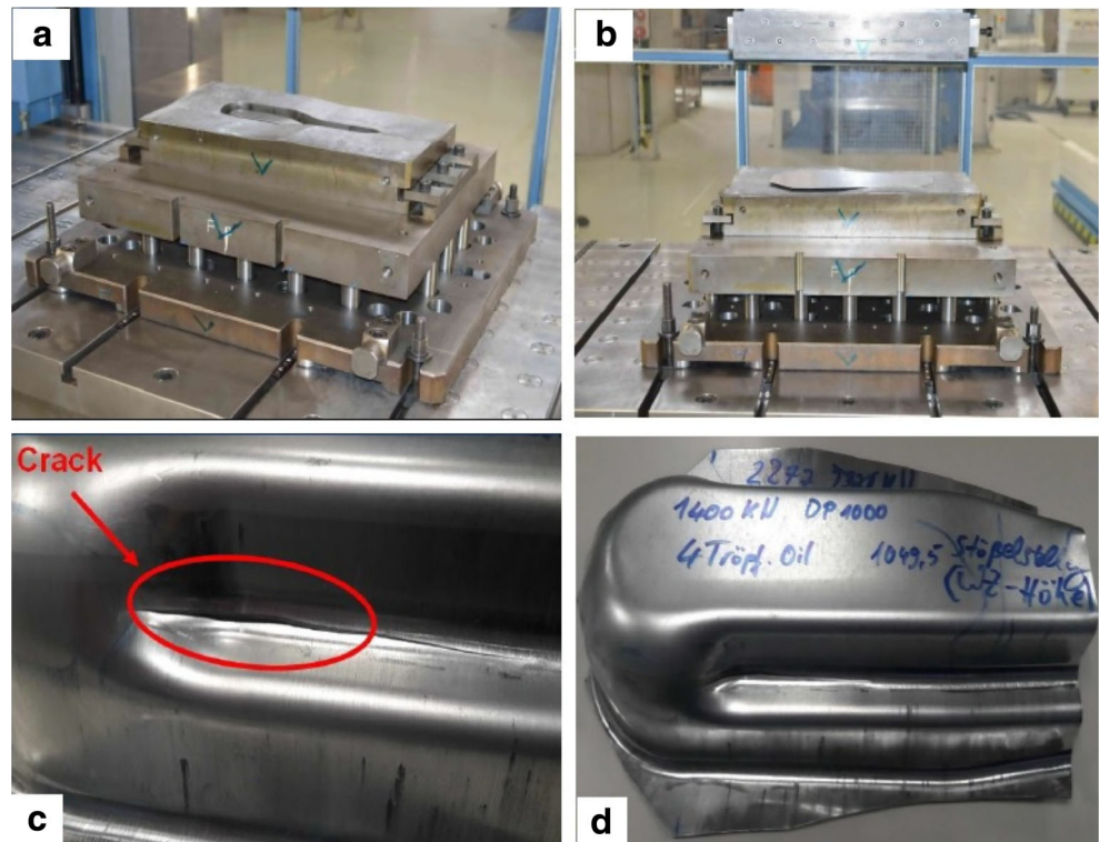
Fig. 11 Setup of stamping test of mini-tunnel sample: (a), (b) used die set and (c), (d) formed sample at failure
