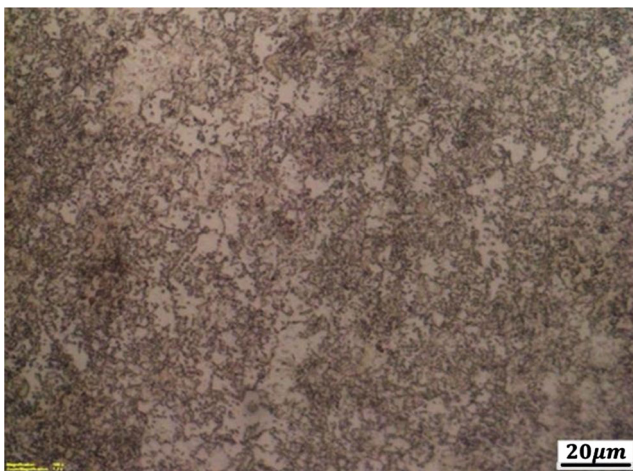
Fig. 1 Micrograph of the investigated steel grade 980
