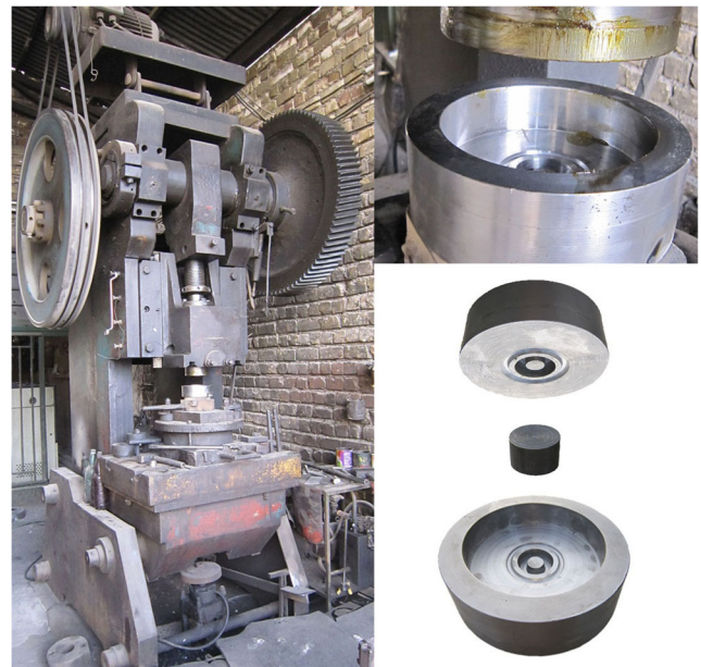
Fig. 8 Configuration of dies assembly for closed hot die forging of case c3
