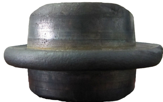
Fig. 9 The experimental forged sample of case c3
