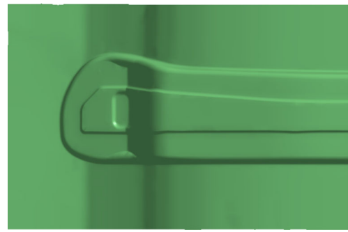
Fig. 15 The illumination map of compensated die mesh
