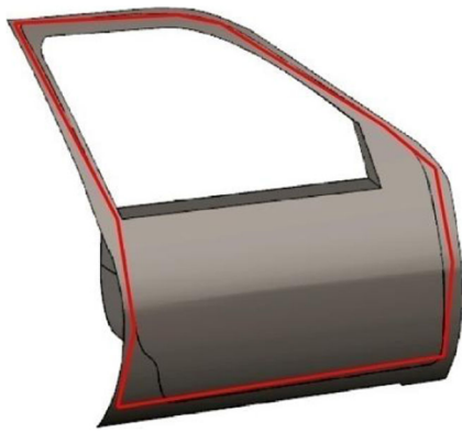
Fig. 1 The edges of automobile panel ( red colour ) which are subjected to bending/hemming operations
