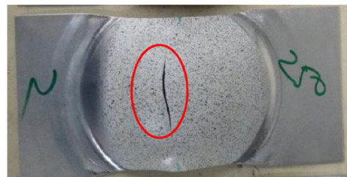
Fig. 5 Failure zone in experimental sample
