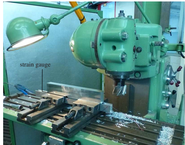
Fig. 3 The experimental set-up used to perform the layer removal method
