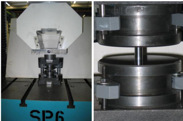
Fig. 4 Experimental setup for the upsetting tests on the universal testing machine
