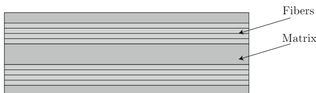
Fig. 1 Composite laminate made of unidirectional prepreps separated by a pure matrix fluid
