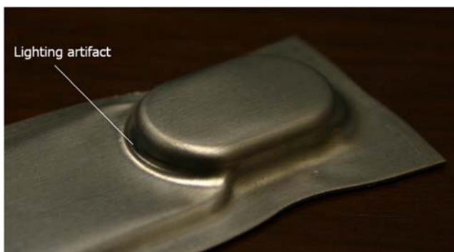
Fig. 10 Forming using Teflon sheet as lubricant, 6.72 kN clamping force, heated dies at 300°C and cold punch at 15°C
