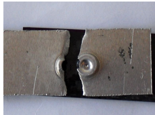
Fig. 10 Particular of the crack in the aluminium alloy
