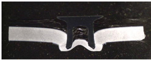
Fig. 5 The transverse section of riveted joints
