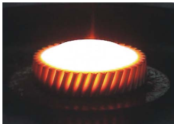
Figure 6: Inhomogeneous cool down of forging
