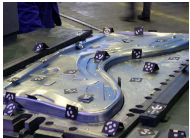
Fig. 4 Formed part prepared for measurement. Bar-coded markers allow multiple camera shots to be overlapped and combined
