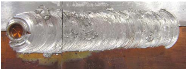
Fig. 15 Final result of the welding of two plates composed by Al 1050 and Cu b1
