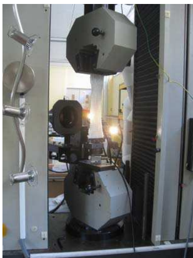
Fig. 2. Bias-extension test setup with image processing tools at INSA-Lyon
