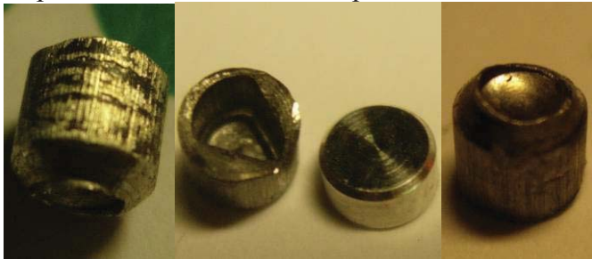
Fig. 7 Left: Formed component at 20°C with cracks in the skirt Right: Billet and formed component at 400°C
