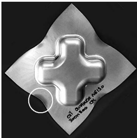
Figure 4: Shiny spots on the blank reveal high-pressure zones (picture courtesy of Corus RD&T)
