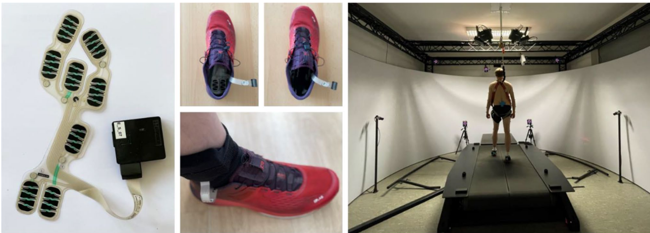
Fig. 1 Body-attached sensor networks (BASN) consisting of a sensor node and a pressure insole, and a participant walking in the Gait Real-time Analysis Interactive Lab (GRAIL). The pressure sensors
